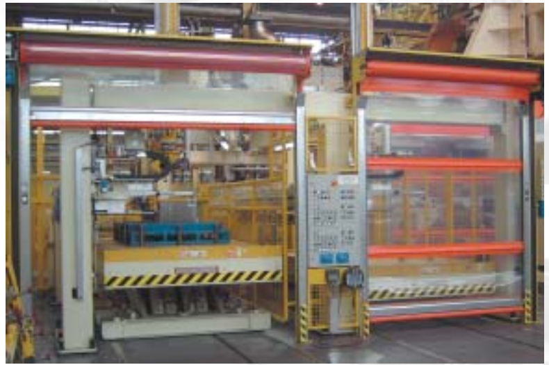
Pallet lift cart and fanner station
