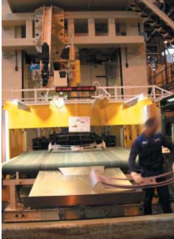
End of line conveyor
